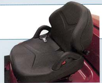
Safer seat with side restraint support
