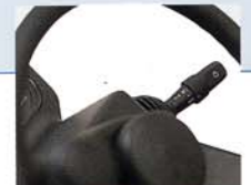
Integrated lights switch
