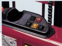
Balance monitoring indicator
