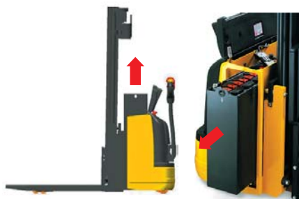
CNI battery removal
